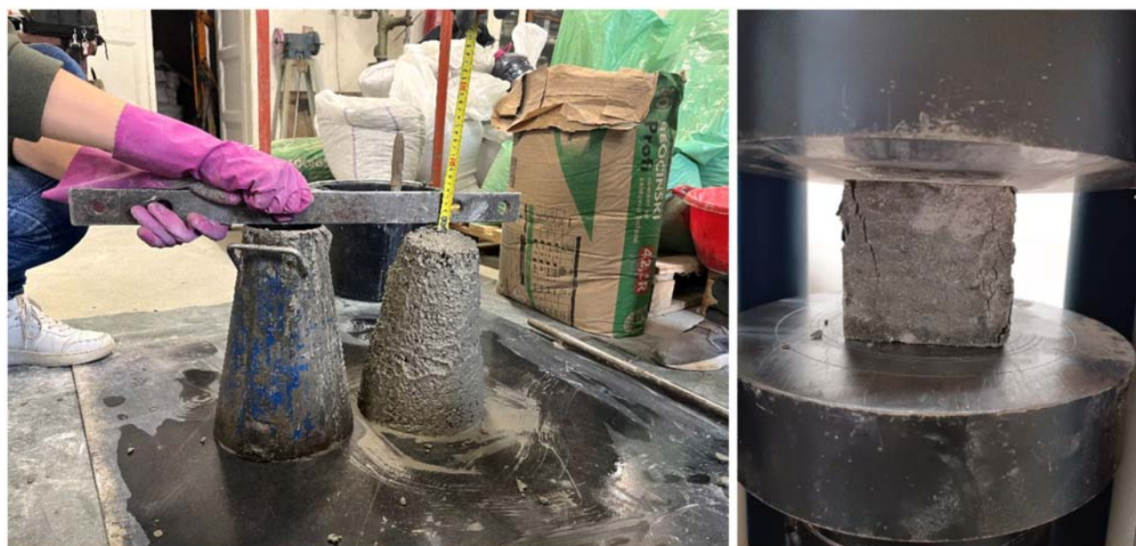
Figure 3.3-41 - Concrete workability testing (left), and compressive strength testing (right)
