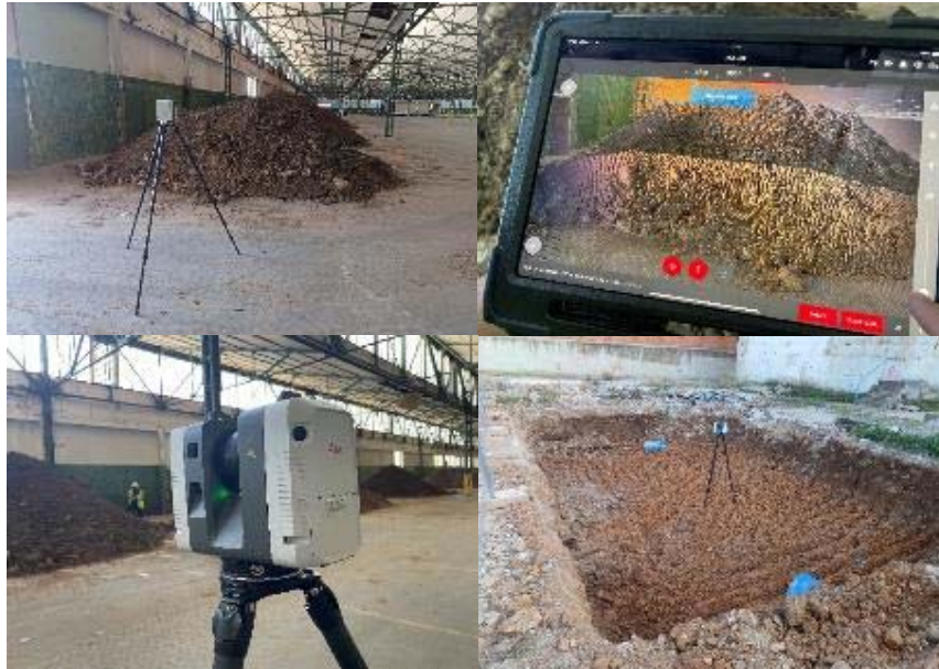
Figure 3.1-8 - Point cloud scanning of the excavated material
