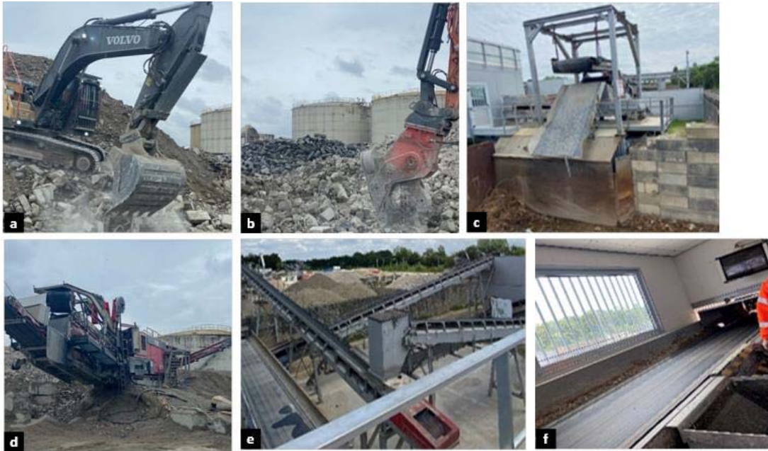
Figure 11 Photos of equipment used in recycling platforms, A: Gripper loader, B: Rock breaker, C: Magnetic conveyor, D: Crusher, E: Screening machine with granulometric material separation belt, F: Sorting belt.
