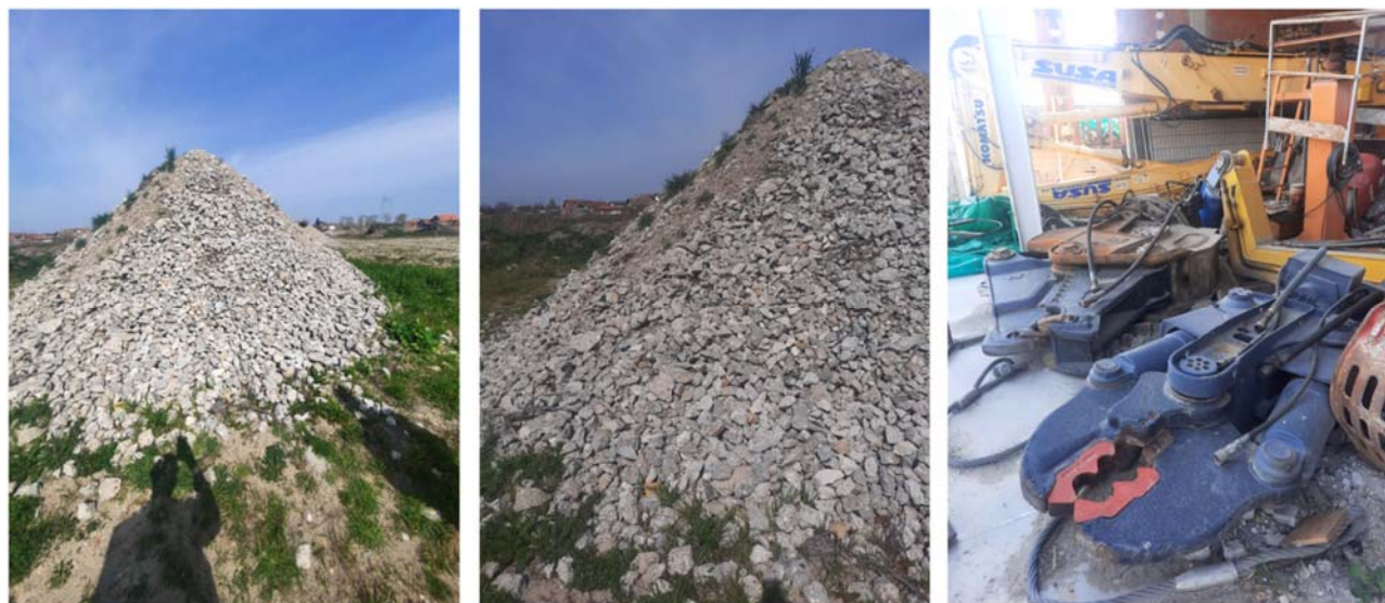
Figure 3.3-34 - Šuša Company, Novi Sad-Recycled concrete aggregate and jaw crusher
