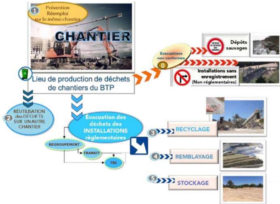
Figure1 general diagram of inert waste flows from construction sites and their treatment channels (Déchets de chantiers du BTP-ORDEEC, 2019)
