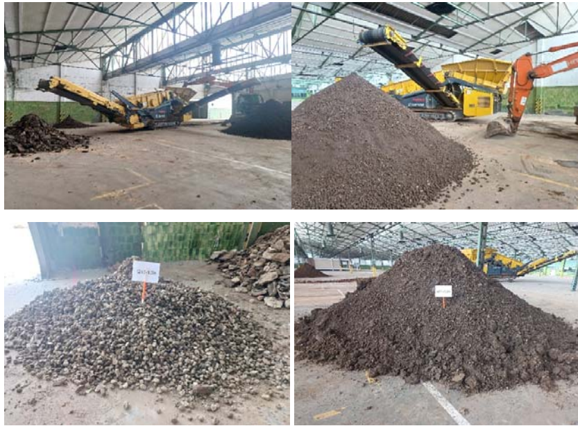
Figure 3.1-4 - Sieving of the material from the five sample sites
