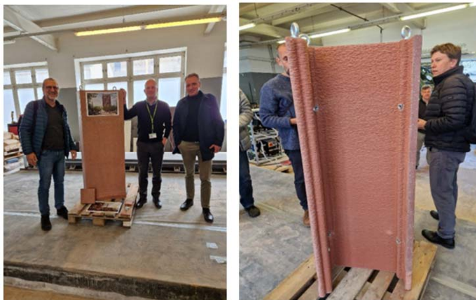
Figure 3.5-2 - Phasade panel demonstrator made by company SO Concrete a.s.: a) presentation on premise of So Concrete; b) detail of anchoring points in the panel
