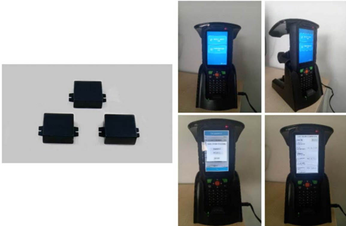
Figure 3.1-10 - RFID sensors selected for application (left) and reader (right)
