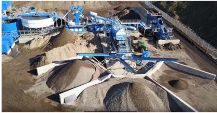
Figure13 (a) All-in-one impact crusher/screener capable of going on site - 2000 t of 20/60 and 0/31.5 aggregates produced per day on site (Groupe Garonne https://www.groupegaronne.fr/le-recyclage-des-deblais-de-chantier/ ), (b) mobile but permanent installation on the Wiame platform with crusher (in yellow) fed by mechanical shovel, then screener/sizer (in blue) with ferrous metal separation and air separator. (c) permanent installation of a recycling platform (Yprema - https://www.yprema.fr/ ), permanent platform with advanced washing treatment and materials collection (CDE - https://www.cdegroupp.com/fr/applications/recyclage-des-dechets ).
