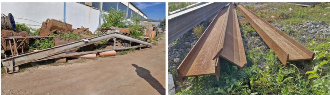
Figure 3.3-37 - Steel components suitable for reuse
