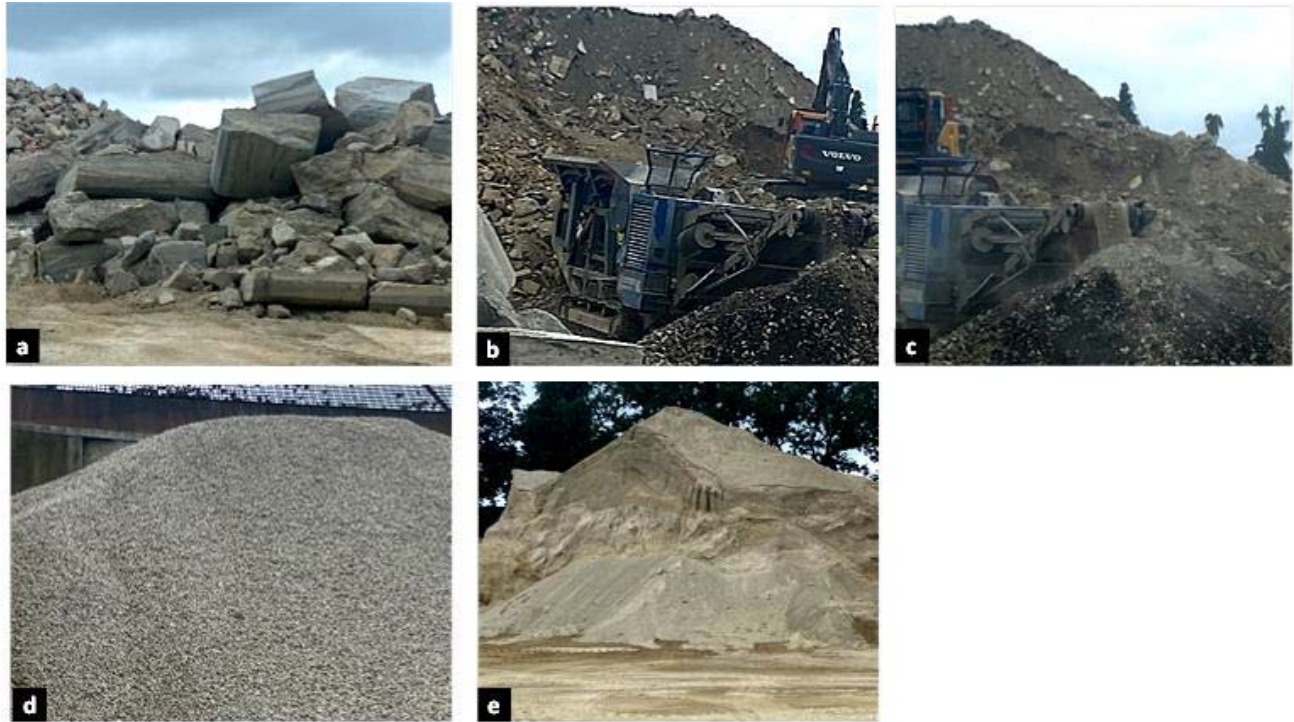
Figure 20 Photograph of the ECOSELECT platform at Verne-sur-Seiche, a : materials storage, b and c: crushing, d and e: storage area for recycled materials.
